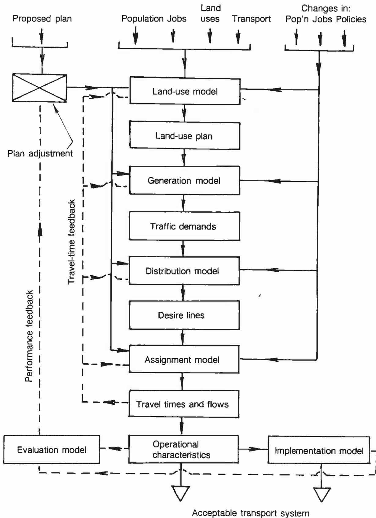
Fig. 2.9 Flow diagram of the interaction land-use and transport planning process
