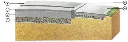
3 The Roman road pavement was based on a compacted earth footing [1] with a layer of small stones in mortar [2] and above this hard filling [3] and a slab surface [4]. At the sides were retaining stones [5] and ditches for drainage [6].
