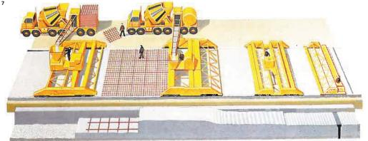
7 Road making is automated in the modern concrete "train". Ready-mixed concrete is fed into a paver which extrudes an even layer as it creeps along. This layer is compacted with poker vibrators. After a mat of steel reinforcing has been laid over the wet concrete a second pave places another laver steel. A vibrating beam is used to compact this thin layer without disturbing the steel.
