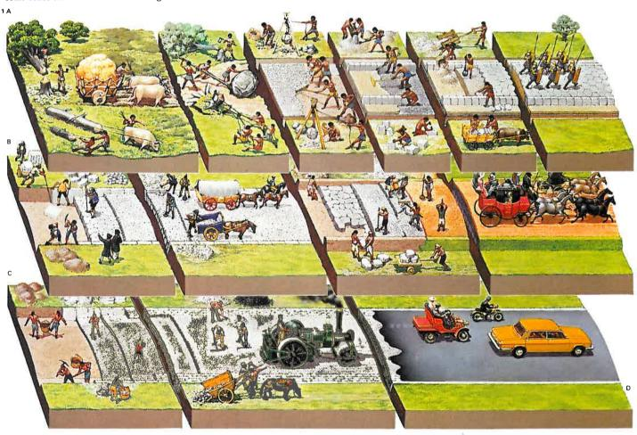
1 Road construction methods grew from simple compaction of early routes by foot and horse-drawn traffic. The Romans [A] made their routes more permanent by removing obstacles, laying foundations of gravel, surfacing with crushed stones or paving slabs and
