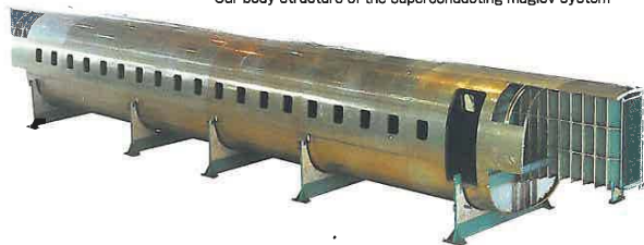
リニア車両用構体 Car body structure of the superconducting maglev system
