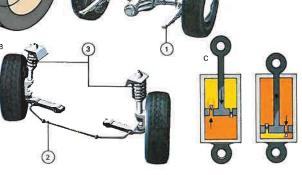
suspension every irregularity of the road surface would be transmitted to the occupants of the car. Springing avoids this problem, but to avoid over-springiness damping must be introduced. [A] shows a rear suspension layout with leaf springs [1] mounted on the axle. The frontwheel suspension [B] shown uses suspension struts [3], which combine coil spring and damper in a single unit, together
