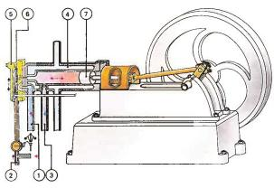
Otto's engine of 1876 was the first successful internal combustion engine. A four-stroke horizontal engine, it used a mixture of gas and air as fuel. The charging stroke drew in air [1] and gas [2] through a slide valve [5] into the cylin-
