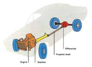
7 The differential enables one of the half-shafts and its road wheel to rotate at a slower rate than the other while the car is turning, even though both sides are being driven. This is necessary when
