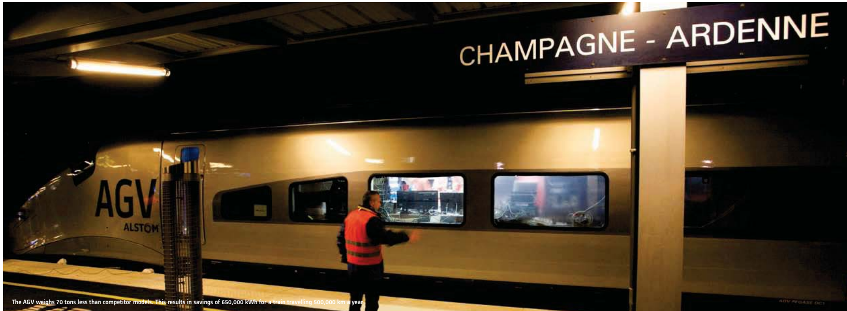
The AGV weighs 70 tons less than competitor models. This results in savings of 650,000 kWh for a train travelling 500,000 km a year.
