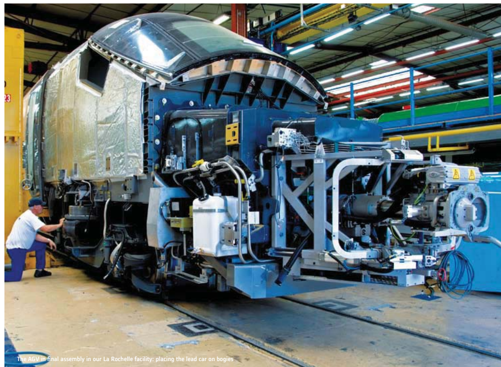
The AGV in final assembly in our La Rochelle facility: placing the lead car on bogies
